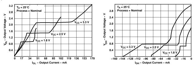
Figure 1. Typical Output Voltage vs Output Current
