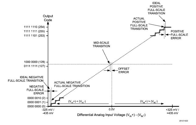
FIGURE 2. Input / Output Transfer Characteristic
