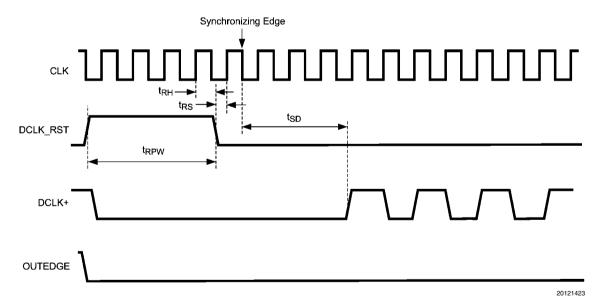
FIGURE 7. Clock Reset Timing in SDR Mode with OUTEDGE Low
