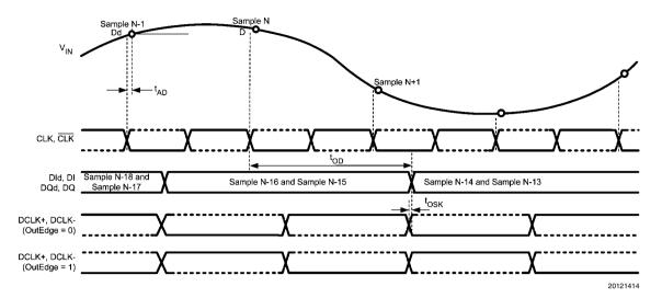
FIGURE 3. ADC08D500 Timing — SDR Clocking
