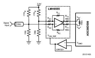
FIGURE 12. Example of Servoing the Analog Input with  $\rm V_{\rm CMO}$
