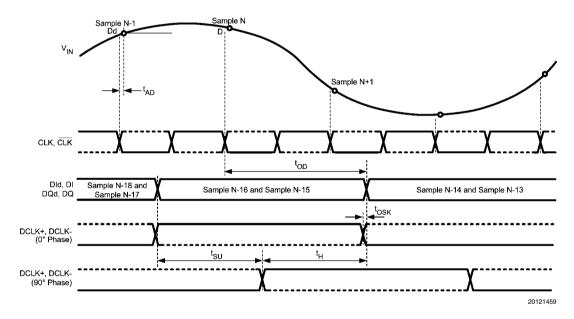
FIGURE 4. ADC08D500 Timing — DDR Clocking
