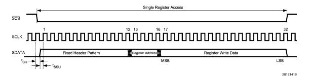
FIGURE 5. Serial Interface Timing
