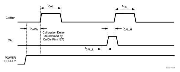
FIGURE 9. Self Calibration and On-Command Calibration Timing
