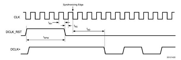
FIGURE 6. Clock Reset Timing in DDR Mode
