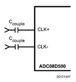
FIGURE 14. Differential (LVDS) Clock Connection
