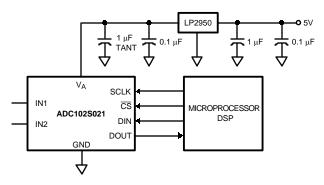
Figure 50. Typical Application Circuit
