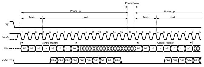
Figure 3. ADC102S021 Operational Timing Diagram
