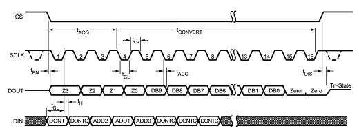
Figure 5. ADC102S021 Serial Timing Diagram
