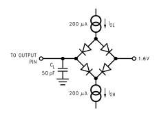
Figure 4. Timing Test Circuit
