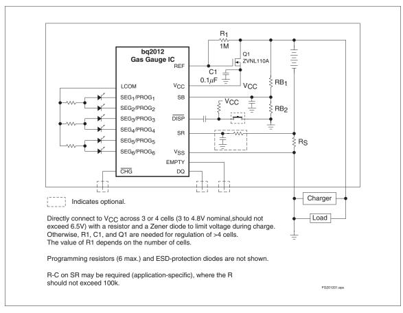
Figure 1. Battery Pack Application Diagram—LED Display
