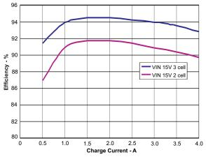
Figure 16. Efficiency vs Output Current (VIN = 15V)
