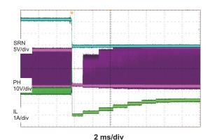
Figure 14. Battery to Ground Short Protection
