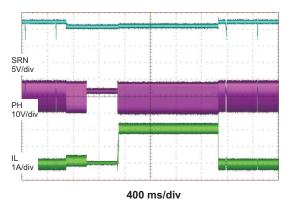
Figure 13. Battery Insertion and Removal
