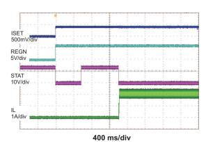
Figure 6. Charge Enable by ISET
