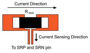
Figure 27. Sensing Resistor PCB Layout
