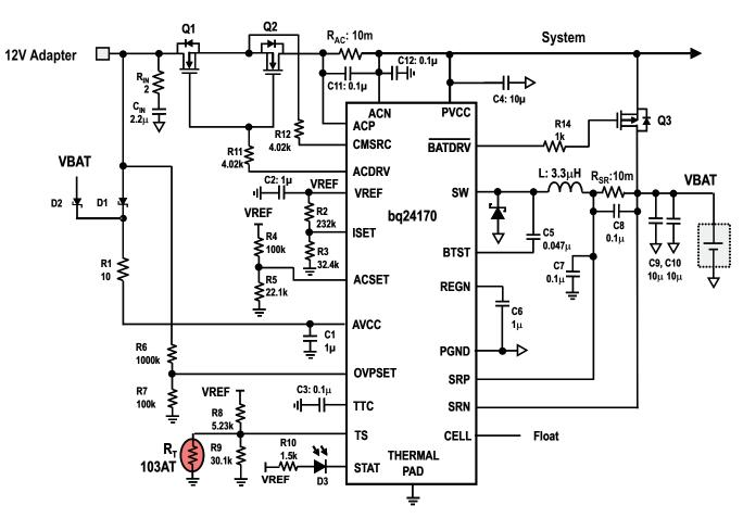
Figure 1. Typical Application Schematic (12V input, 2 cell battery 8.4V, 2A charge current, 0.2A pre-charge/termination current, 3A DPM current, 18V input OVP, 0 – 45°C TS)
