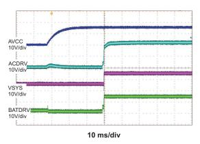
Figure 11. BATFET to ACFET Transition During Powerup
