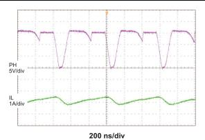
Figure 10. Discontinuous Conduction Mode Switching
