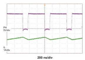
Figure 9. Continuous Conduction Mode Switching
