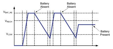
Figure 21. Battery Detect Timing Diagram
