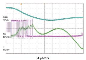
Figure 15. Battery to Ground Short Transition
