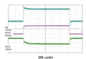
Figure 12. System Load Transient (Input current DPM)
