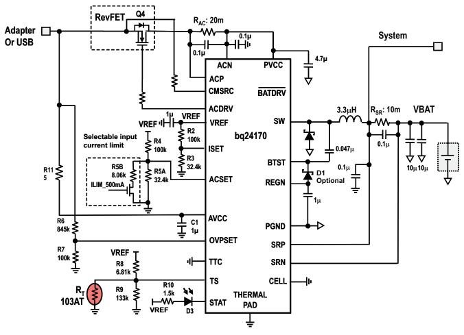
Figure 3. Typical Application Schematic wth Single Cell Unremovable Battery (USB or adapter with input OVP 15V, up to 4A charge current, 0.4A pre-charge current, 2A adapter current or 500mA USB current,  $5-40^{\circ}\text{C}$  TS, system connected before sense resistor)
