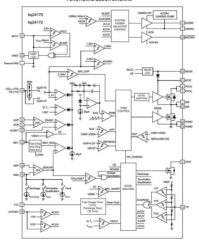
Figure 18. Functional Block Diagram
