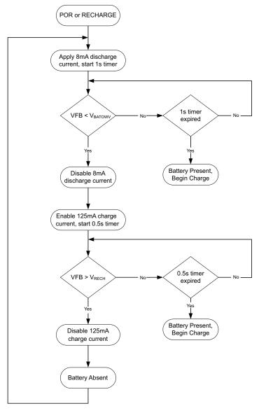
Figure 20. Battery Detection Flowchart
