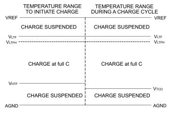
Figure 22. TS Pin, Thermistor Sense Thresholds
