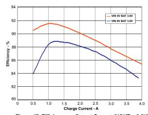
Figure 17. Efficiency vs Output Current (VOUT = 3.8V)
