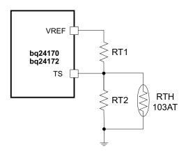
Figure 23. TS Resistor Network
