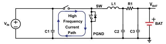
Figure 26. High Frequency Current Path
