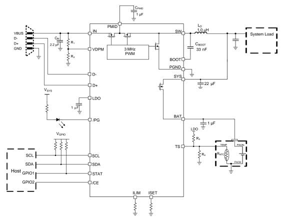
Figure 29. bq24251 Typical Application Circuit
