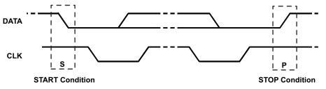
Figure 25. START and STOP Condition
