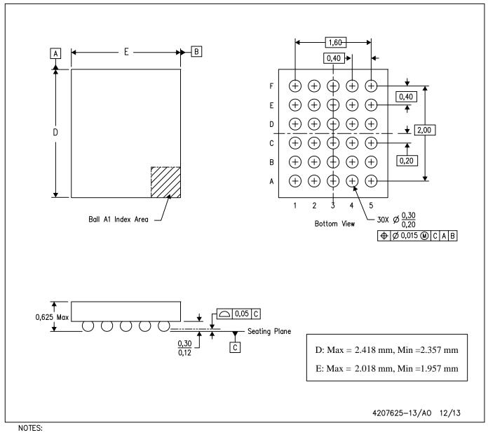
A. All linear dimensions are in millimeters. Dimensioning and tolerancing per ASME Y14.5M-1994.
