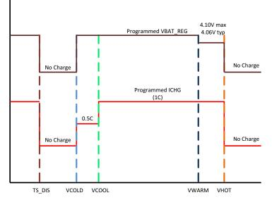
Figure 23. JEITA Profile for Voltage and Current Regulation Loops
