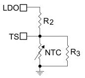
Figure 21. Voltage Based NTC Circuit
