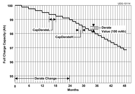
Figure 1. Age Based Capacity Method
