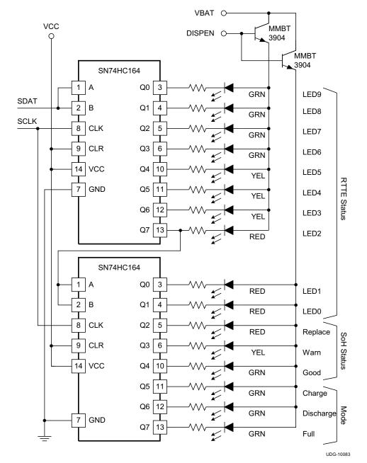
Figure 2 shows the application schematic showing the 10-bar LED bar graph display and status LED connections.
