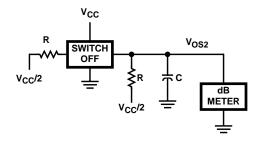
FIGURE 4. CROSSTALK BETWEEN TWO SWITCHES TEST CIRCUIT
