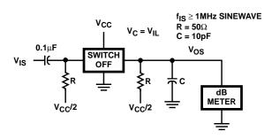
FIGURE 7. CONTROL-TO-SWITCH FEEDTHROUGH NOISE TEST CIRCUIT
