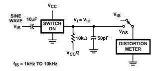
FIGURE 5. FREQUENCY RESPONSE TEST CIRCUIT
