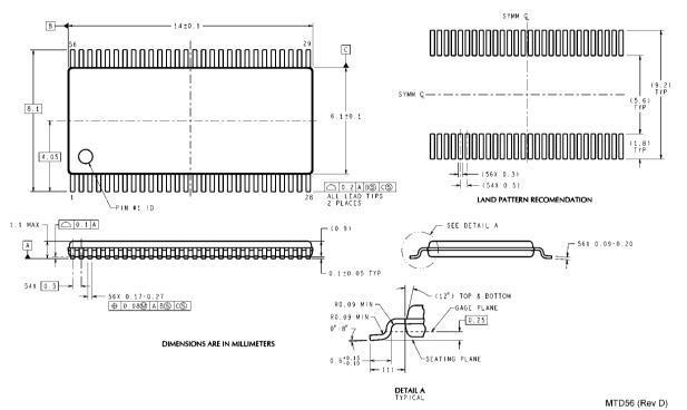
56-Lead Molded Thin Shrink Small Outline Package, JEDEC Dimensions shown in millimeters only Order Number DS90CR286AMTD, DS90CR286AQMT NS Package Number MTD56
