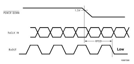
FIGURE 8. DS90CR286A/DS90CR216A (Receiver) Power Down Delay
