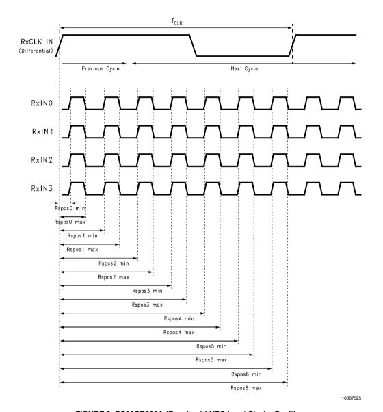
FIGURE 9. DS90CR286A (Receiver) LVDS Input Strobe Position
