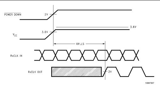
FIGURE 5. DS90CR286A/DS90CR216A (Receiver) Phase Lock Loop Set Time
