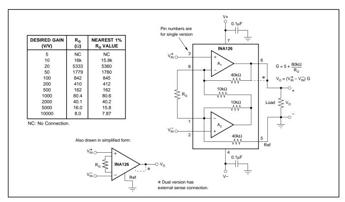
FIGURE 1. Basic Connections.
