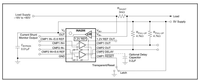
Figure 30. INA20x Basic Connection
