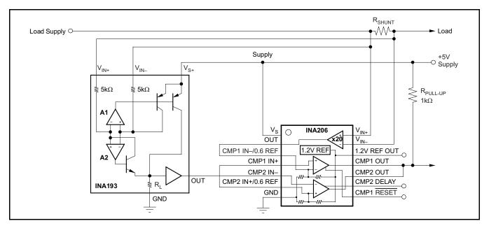
Figure 40. Bi-Directional Current Comparator
