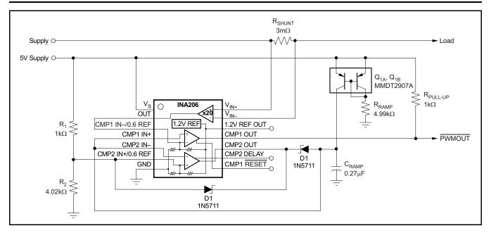
Figure 39. PWM Output Current-Shunt Monitor
