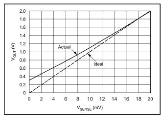
Figure 31. Example for Low V<sub>SENSE</sub> Cases 1 and 3 (INA208, Gain = 100)
