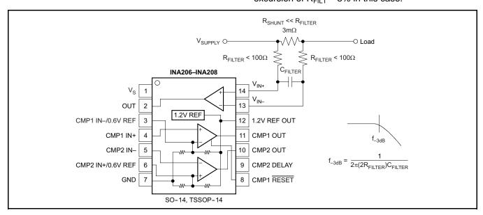
Figure 33. Input Filter (Gain Error -1.5% to -2.2%)
