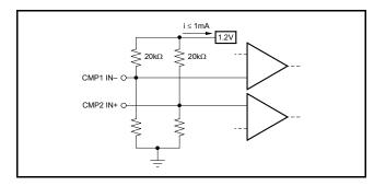
Figure 37. Limit Current Into Reference ≤ 1mA
