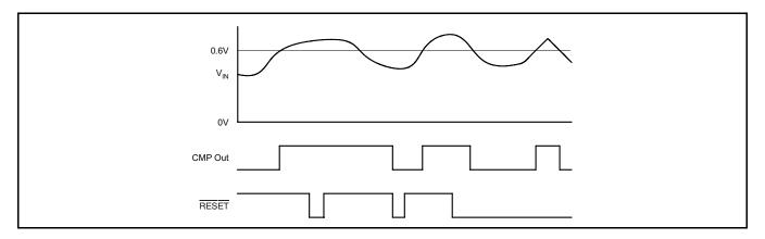
Figure 35. Comparator 1 Latching Capability
