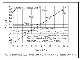
Figure 32. Example for Low V<sub>SENSE</sub> Case 2 (INA208, Gain = 100)
