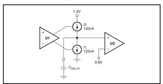
Figure 34. Simplified Model of the Comparator 2
