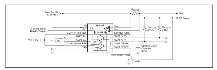
Figure 38. Overdriving Comparator Inputs Without Generating a Reference Error
