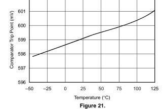
**COMPARATOR TRIP POINT vs TEMPERATURE**
