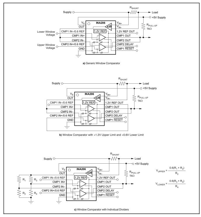
Figure 41. Using the INA206, INA207, and INA208 as Window Comparators
