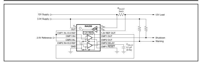
Figure 36. Server 12V Supply Current Monitor
