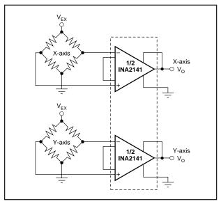
FIGURE 4. Two-Axis Bridge Amplifier.
