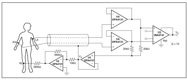
FIGURE 6. ECG Amplifier With Right-Leg Drive.
