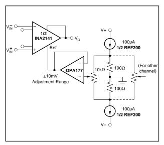
FIGURE 2. Optional Trimming of Output Offset Voltage.
