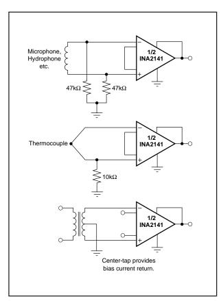
FIGURE 3. Providing an Input Common-Mode Current Path.
