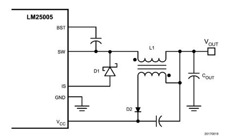
FIGURE 13. VCC Bias with Additional Winding on the Output Inductor
