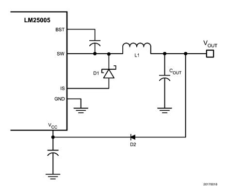
FIGURE 12. VCC Bias from VOUT for 8V < VOUT < 14V
