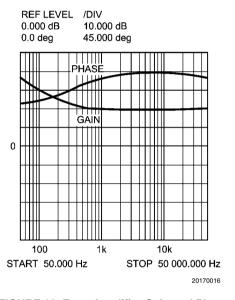
FIGURE 10. Error Amplifier Gain and Phase
