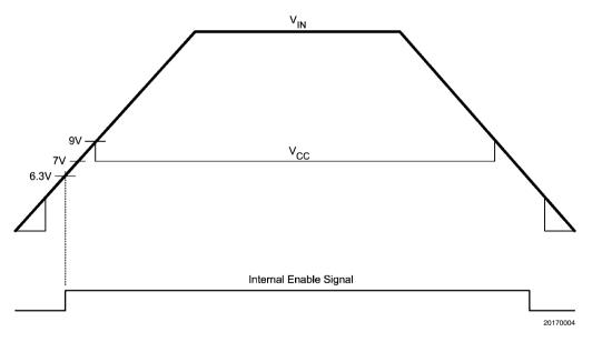
FIGURE 2. Vin and Vcc Sequencing
