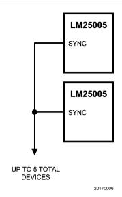
**FIGURE 4. Sync from Multiple Devices**
