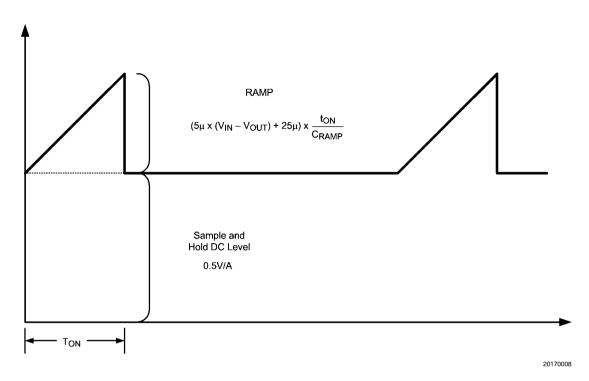
FIGURE 6. Composition of Current Sense Signal
