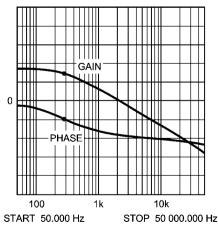
FIGURE 9. Gain and Phase of Modulator  $R_{LOAD} = 5$  Ohms and  $C_{OUT} = 177 \mu F$
