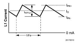
FIGURE 8. Inductor Current Waveform
