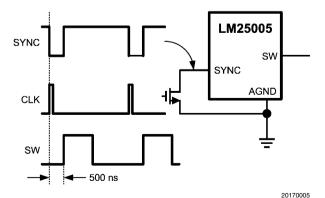
FIGURE 3. Sync from External Clock
