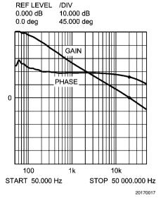
FIGURE 11. Overall Loop Gain and Phase
