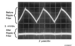
FIGURE 20. Post Ripple Filter Waveform
