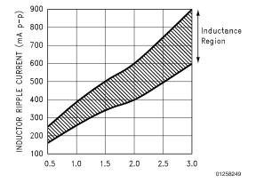
FIGURE 21. Peak-to-Peak Inductor Ripple Current vs Load Current
