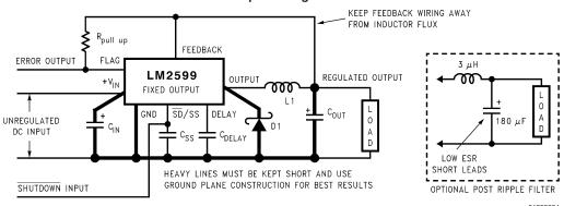
Component Values shown are for  $V_{\mbox{\footnotesize{IN}}}$  = 15V,
