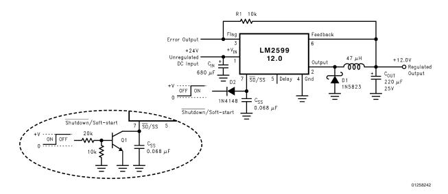
FIGURE 26. Typical Circuit Using Shutdown /Soft-start and Error Flag Features
