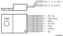
Order Number LM2599T-3.3, LM2599T-5.0, LM2599T-12 or LM2599T-ADJ See NS Package Number TA07B Surface Mount Package 7-Lead TO-263 (S)
