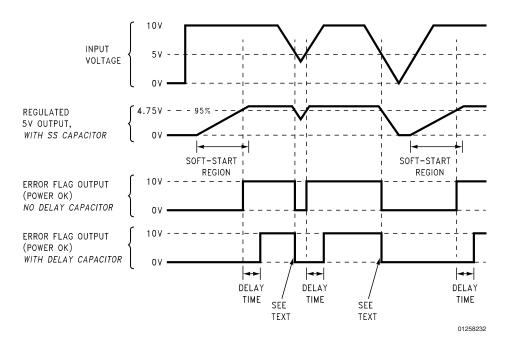
FIGURE 14. Timing Diagram for 5V Output
