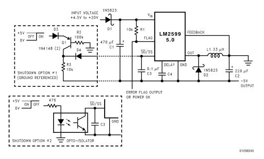
FIGURE 27. Inverting -5V Regulator With Shutdown and Soft-start
