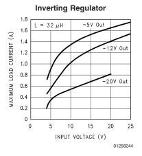
FIGURE 28. Maximum Load Current for Inverting Regulator Circuit
