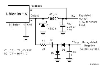
FIGURE 32. Charge Pump for Generating a Low Current, Negative Output Voltage
