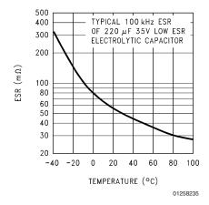
FIGURE 18. Capacitor ESR Change vs Temperature
