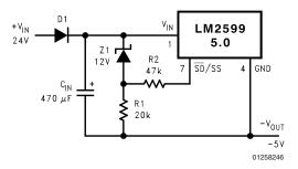
FIGURE 31. Undervoltage Lockout With Hysteresis for an Inverting Regulator
