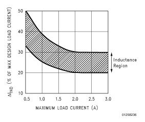
FIGURE 19. (△I<sub>IND</sub>) Peak-to-Peak Inductor Ripple Current (as a Percentage of the Load Current) vs Load Current
