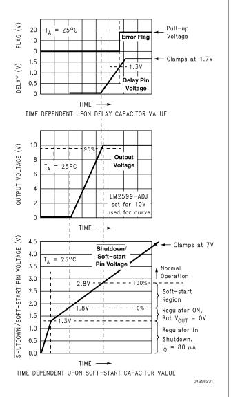
FIGURE 13. Soft-start, Delay, Error, Output
