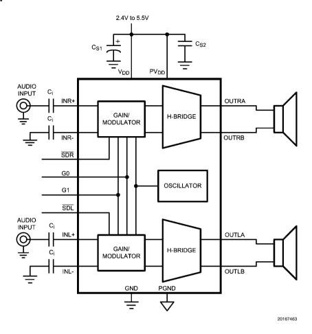
$C_i = 1 \mu F$   $C_{S1} = 1 \mu F$  $C_{S2} = 0.1 \mu F$
