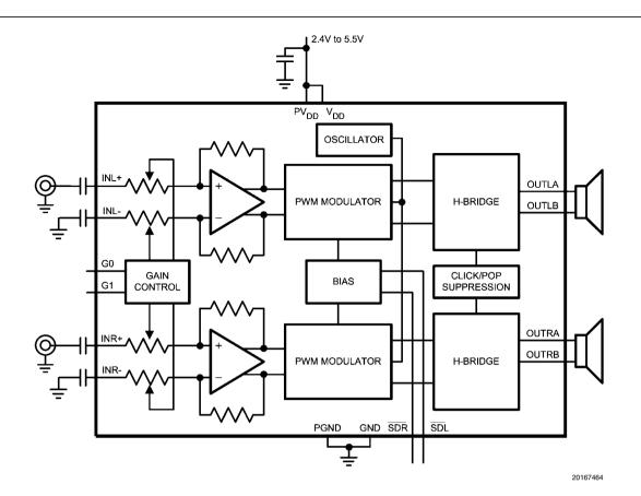
FIGURE 3. Single-Ended Input Configuration
