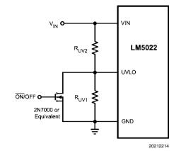
FIGURE 2. Enable/Disable Using UVLO
