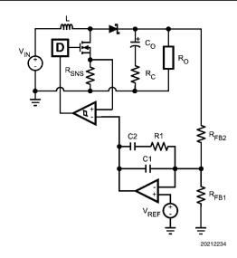
FIGURE 7. Power Stage and Error Amp
