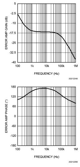
FIGURE 9. Error Amplifier Gain and Phase
