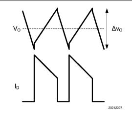
FIGURE 6. ΔV<sub>o</sub> Using Low ESR Capacitors
