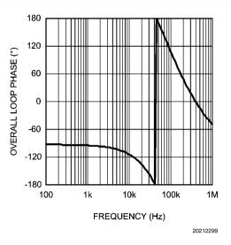
FIGURE 10. Overall Loop Gain and Phase
