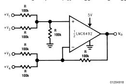
Where:  $V_0 = V_1 + V_2 - V_3 - V_4$  $(V_1 + V_2 \ge (V_3 + V_4) \text{ to keep } V_0 > 0V_{DC}$
