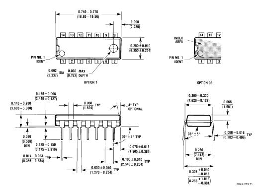
14-Lead Molded Dual-In-Line Package
