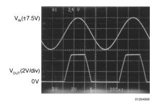
FIGURE 2. A ±7.5V Input Signal Greatly Exceeds the 5V Supply in *Figure 3* Causing No Phase Inversion Due to R<sub>I</sub>
