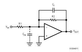
FIGURE 4. Cancelling the Effect of Input Capacitance
