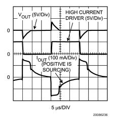
FIGURE 2. V<sub>COM</sub> Output, High Current Drive Waveform, & LMH6640 Output Current Waveforms
