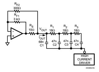
FIGURE 1. LMH6640 in a V<sub>COM</sub> Buffer Application with Simulated TFT Load
