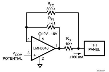
Typical Application as a TFT Panel V<sub>COM</sub> Driver
