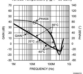
Gain vs. Frequency Normalized  $(P_{IN}=-30dBm)$
