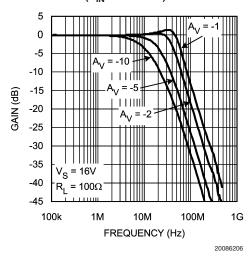
Gain vs. Frequency for Various V<sub>S</sub>  $(P_{IN} = -30 \text{ dBm})$
