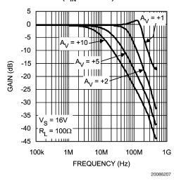
Gain vs. Frequency for Various V<sub>S</sub>  $(P_{IN} = -30 \text{ dBm})$
