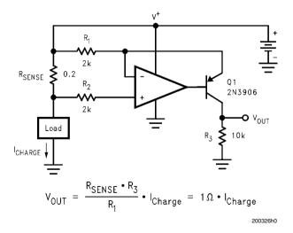
FIGURE 2. High Side Current Sensing
