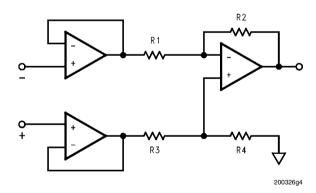
FIGURE 5. Rail-to-rail Instrumentation Amplifier
