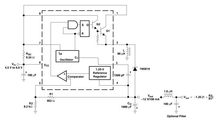
Figure 10. Voltage-Inverting Converter
