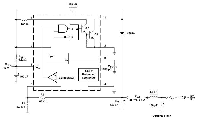
Figure 6. Step-Up Converter
