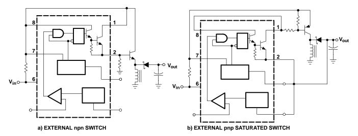
Figure 11. External Current-Boost Connections for I<sub>C</sub> Peak Greater Than 1.5 A
