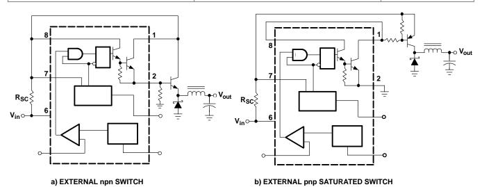
Figure 9. External Current-Boost Connections for I<sub>C</sub> Peak Greater Than 1.5 A
