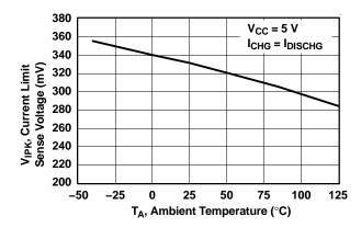
Figure 4. Current-Limit Sense Voltage vs Temperature
