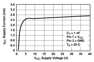
Figure 5. Standby Supply Current vs Supply Voltage
