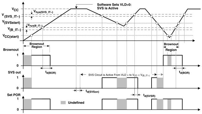
Figure 9. SVS Reset (SVSR) vs Supply Voltage
