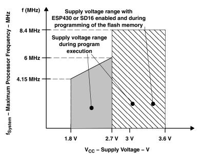
Figure 1. Frequency vs Supply Voltage
