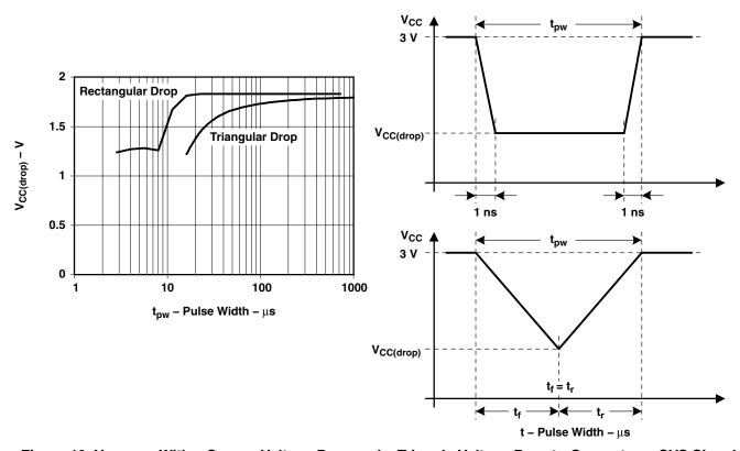
Figure 10. V<sub>CC(drop)</sub> With a Square Voltage Drop and a Triangle Voltage Drop to Generate an SVS Signal
