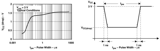
Figure 7. V<sub>CC(drop)</sub> Level With a Square Voltage Drop to Generate a POR/Brownout Signal
