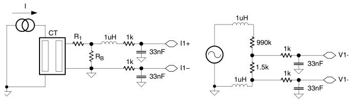
Figure 14. Energy Measurement Test Circuitry (SD16GAINx = 1)
