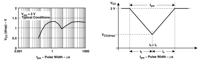
Figure 8. V<sub>CC(drop)</sub> Level With a Triangle Voltage Drop to Generate a POR/Brownout Signal
