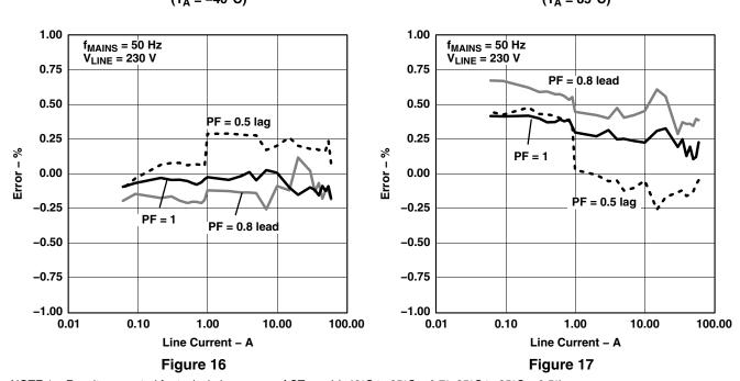
NOTE 1: Results corrected for typical phase error of CT used ( $-40^{\circ}$ C to 25°C:  $-0.7^{\circ}$ ; 25°C to 85°C:  $+0.5^{\circ}$ ). See Figure 14 for test circuitry: CT part number = T60404-E4624-X101 ( Vacuumschmelze), R<sub>1</sub> = 0  $\Omega$ , R<sub>B</sub> = 12.4  $\Omega$ .
