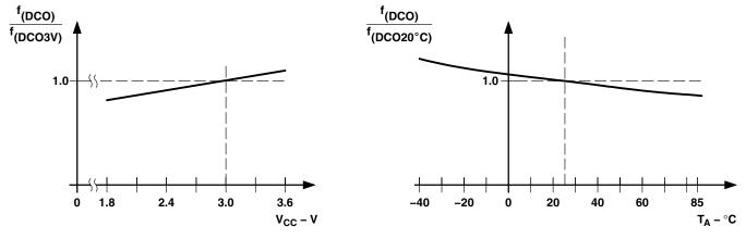
Figure 11. DCO Frequency vs Supply Voltage  $V_{\text{CC}}$  and vs Ambient Temperature
