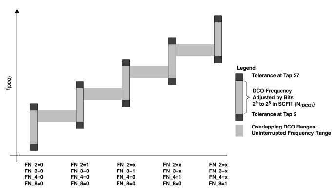
Figure 13. Five Overlapping DCO Ranges Controlled by FN\_x Bits
