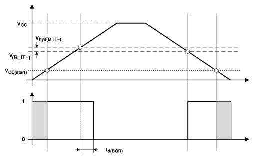
Figure 6. POR/Brownout Reset (BOR) vs Supply Voltage
