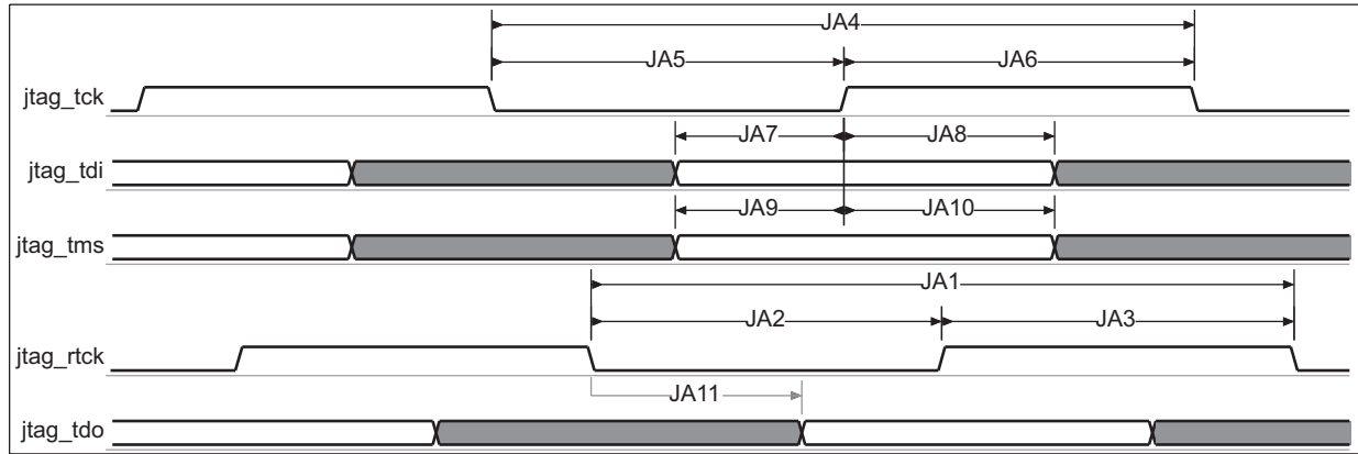
Figure 6-73. JTAG Interface Timing – Adaptive Clock Mode
