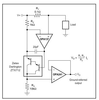
FIGURE 2. High-Side Current Monitor.
