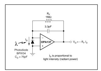
FIGURE 3. Photodetector Amplifier.
