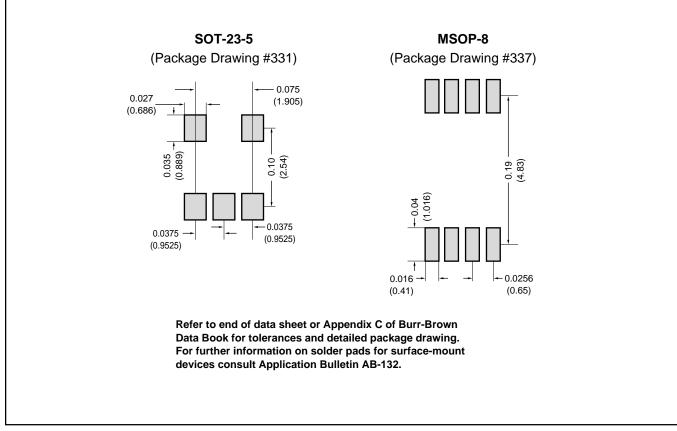
FIGURE 4. Recommended SOT-23-5 and MSOP-8 Solder Footprints.
