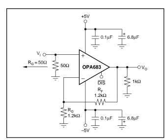
FIGURE 1. DC-Coupled, G = +2V/V, Bipolar Supply, Specification and Test Circuit.
