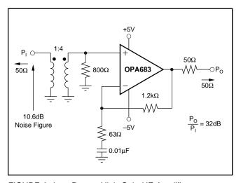
FIGURE 8. Low Power, High Gain HF Amplifier.
