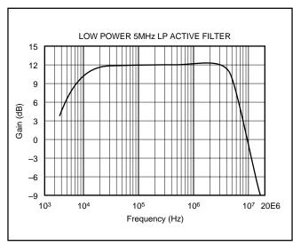
FIGURE 7. Low Power Active Filter Frequency Response.
