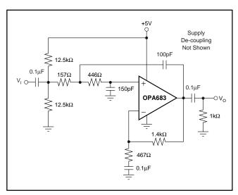
FIGURE 6. 5MHz, 2nd-Order Low Pass Filter.
