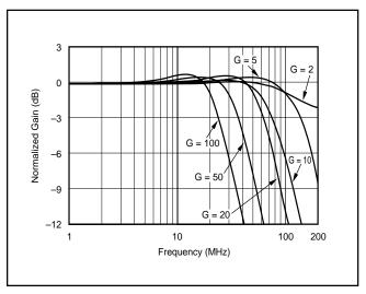
FIGURE 12. Small-Signal Frequency Response with Optimized R<sub>F</sub>.
