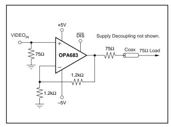
FIGURE 5. Gain of +2 Video Cable Driver.
