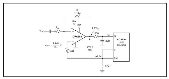
FIGURE 9. Low Power, Single-Supply, ADC Driver.
