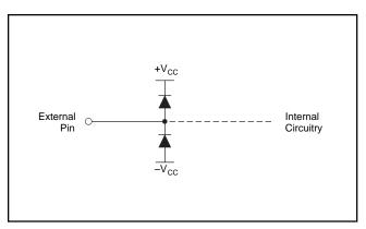
FIGURE 15. Internal ESD Protection.
