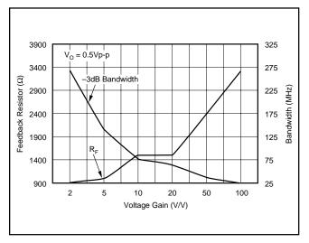
FIGURE 11. Bandwidth and R<sub>F</sub> Optimized vs Gain.
