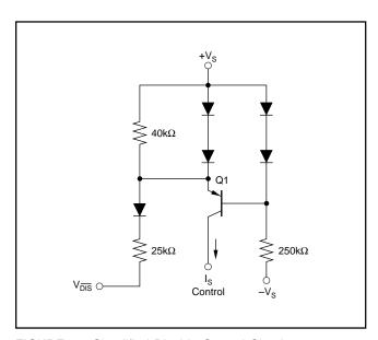
FIGURE 14. Simplified Disable Control Circuit.
