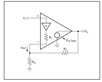
FIGURE 10. Current Feedback Transfer Function Analysis Circuit.
