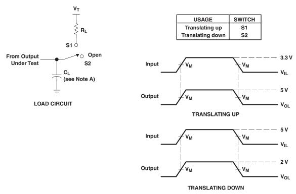
NOTES: A.  $C_L$  includes probe and jig capacitance. B. All input pulses are supplied by generators having the following characteristics: PRR  $\leq$  10 MHz,  $Z_O = 50 \Omega$ ,  $t_f \leq$  2 ns,  $t_f \leq$  2 ns.
