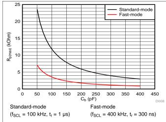
Figure 7. Maximum Pull-up Resistance ( $R_{p(max)}$ ) vs Bus Capacitance ( $C_b$ )
