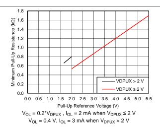
Figure 8. Minimum Pull-up Resistance ( $R_{p(min)}$ ) vs Pull-up Reference Voltage ( $V_{DPUX}$ )
