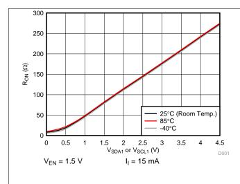
Figure 1. On-Resistance (R<sub>ON</sub>) vs Input Voltage (V<sub>SDA1</sub> or  $V_{SCL1}$ )
