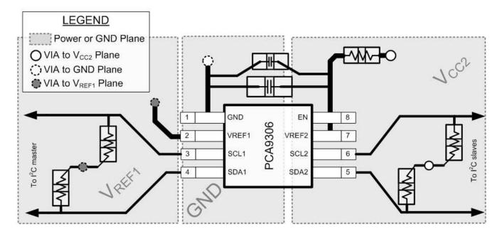
Figure 10. PCA9306 Layout Example
