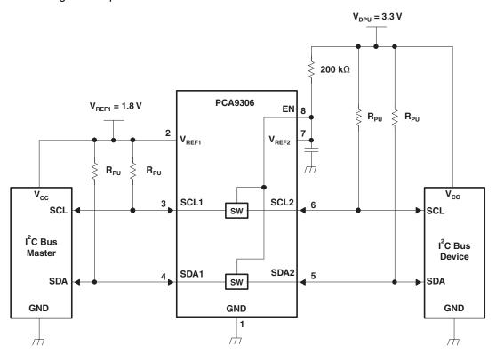
Figure 5. Typical Application Circuit (Switch Always Enabled)
