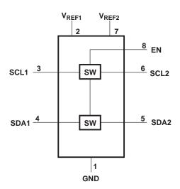
Figure 4. Logic Diagram (Positive Logic)
