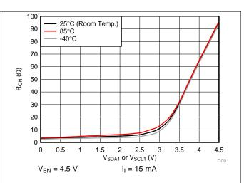
Figure 2. On-Resistance (R<sub>ON</sub>) vs Input Voltage (V<sub>SDA1</sub> or V<sub>SCL1</sub>)
