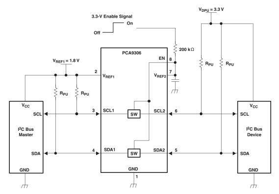
Figure 6. Typical Application Circuit (Switch Enable Control)
