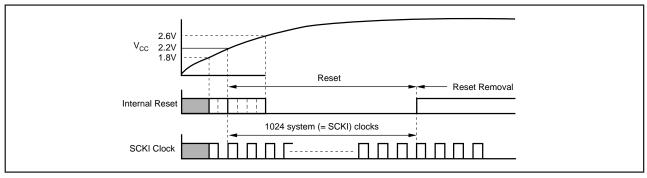
FIGURE 6. Internal Power-On Reset Timing.
