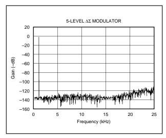
FIGURE 11. Quantization Noise Spectrum.
