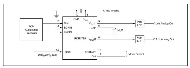
FIGURE 5. Typical Connection Diagram.
