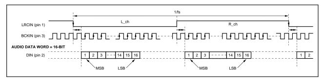
FIGURE 2. "I2S" Data Input Timing.
