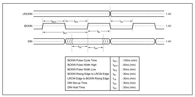
FIGURE 3. Audio Data Input Timing.
