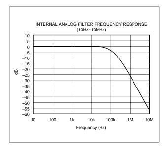
FIGURE 8. Low Pass Filter Wideband Frequency Response.
