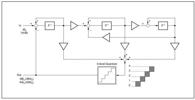
FIGURE 10. 5-Level  $\Delta\Sigma$  Modulator Block Diagram.
