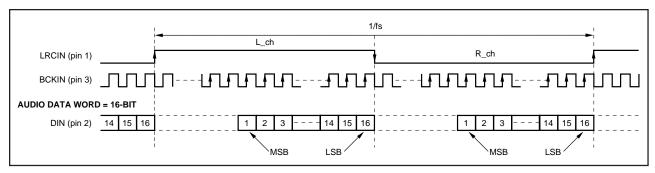
FIGURE 1. "Normal" Data Input Timing.
