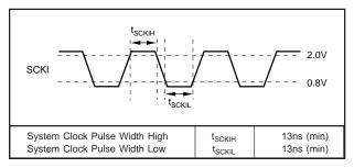
FIGURE 4. System Clock Timing Requirements.
