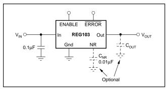
FIGURE 1. Fixed Voltage Nominal Circuit for REG103.
