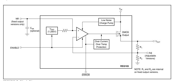
FIGURE 7. Block Diagram.
