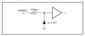
FIGURE 4. ENABLE Pin Equivalent Input Circuit.
