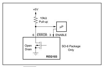
FIGURE 6. ERROR Pin Typical Fault-Monitoring Circuit.
