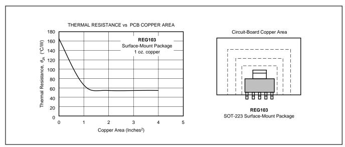
FIGURE 13. Thermal Resistance versus PCB Area for the Five-Lead SOT-223.
