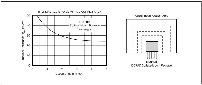
FIGURE 12. Thermal Resistance versus PCB Area for the Five-Lead DDPAK.
