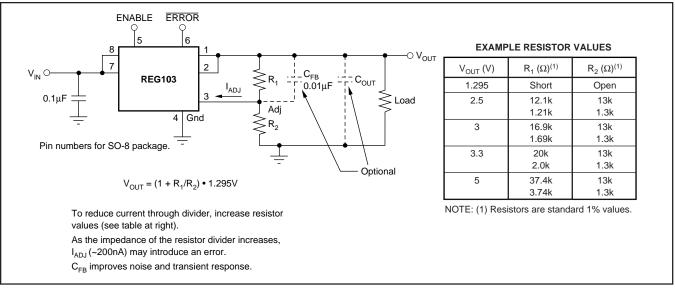
FIGURE 2. Adjustable Voltage Circuit for REG103A.
