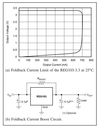
FIGURE 3. Foldback Current Limit and Boost Circuit.
