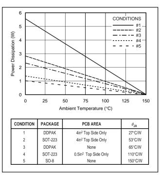
FIGURE 11. Maximum Power Dissipation versus Ambient Temperature for the Various Packages and PCB Heat Sink Configurations.
