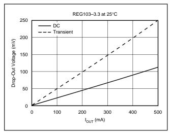
FIGURE 10. Transient and DC Dropout.
