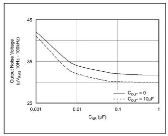
FIGURE 8. Output Noise versus Noise-Reduction Capacitor.
