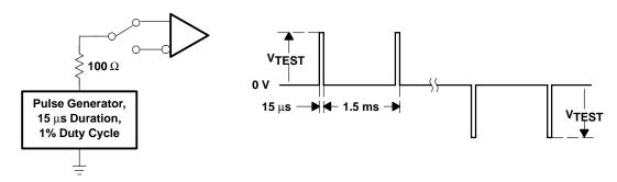
Figure 5. Test Circuit and Waveform, Transient Over-Voltage Test
