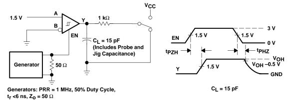
Figure 3. Test Circuit Waveforms, tpzH and tpHZ
