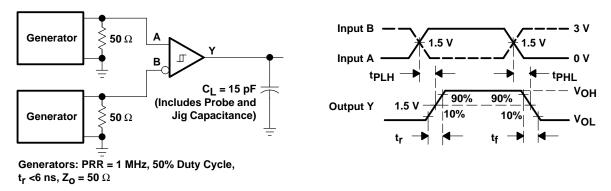
Figure 2. Switching Test Circuit and Waveforms
