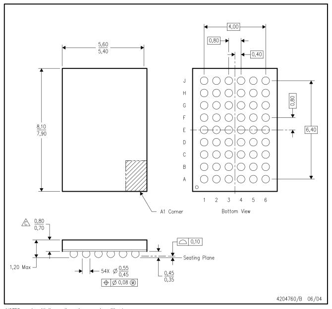
$\hbox{NOTES:} \quad \hbox{A. All linear dimensions are in millimeters.}$
