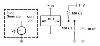
Figure 1. Device Test Setup
