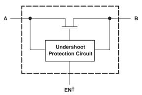
$^{\dagger}$  EN is the internal enable signal applied to the switch.
