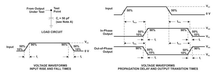
NOTES: A. C<sub>L</sub> includes probe and test-fixture capacitance.
