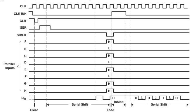
typical clear, shift, load, inhibit, and shift sequence
