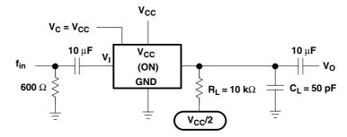
Figure 10. Sine-Wave Distortion
