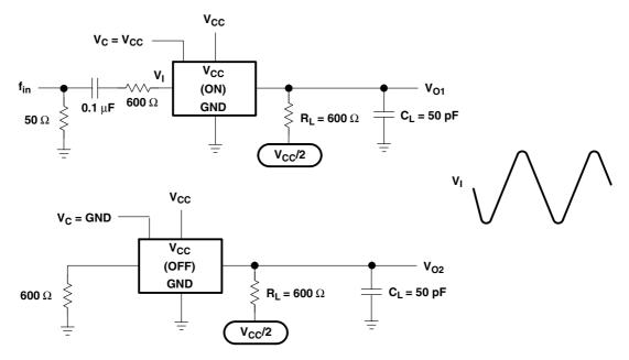
Figure 7. Crosstalk Between Any Two Switches
