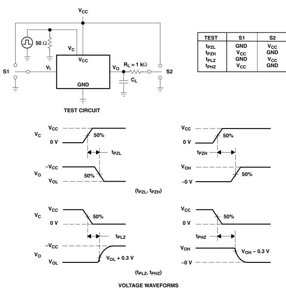
Figure 5. Switching Time (t<sub>PZL</sub>, t<sub>PLZ</sub>, t<sub>PLZ</sub>, t<sub>PHZ</sub>), Control to Signal Output
