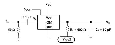
Figure 6. Frequency Response (Switch On)
