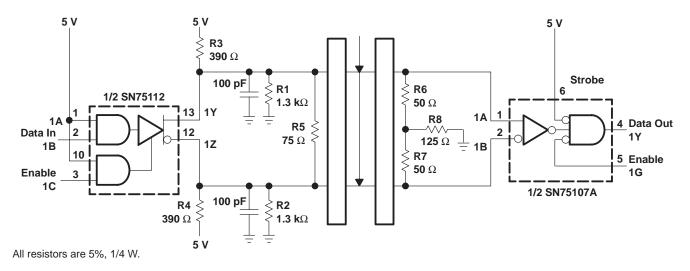
Figure 5. CCITT-Recommended V.35 Interface Using the SN75112 and SN75107A
