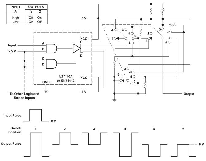
Figure 4. Pulse-Control Circuit
