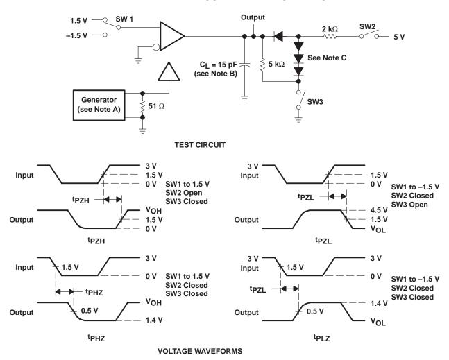
NOTES: A. The input pulse is supplied by a generator having the following characteristics: PRR = 1 MHz, duty cycle = 50%,  $t_{\Gamma} = t_{f} = 6$  ns.
