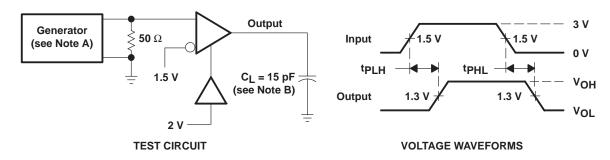
NOTES: A. The input pulse is supplied by a generator having the following characteristics: PRR = 1 MHz, duty cycle = 50%,  $t_f = t_f = 6$  ns.
