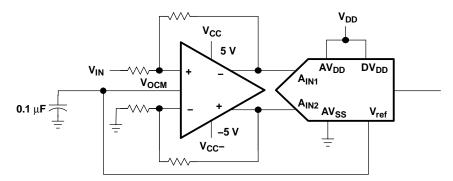
Figure 30. Fully Differential Amplifier Attached to a Differential ADC
