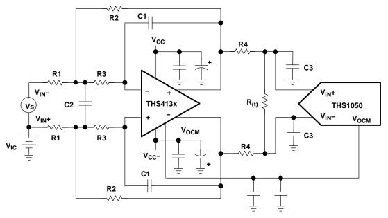
Figure 34. Antialias Filtering
