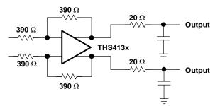
Figure 33. Driving a Capacitive Load
