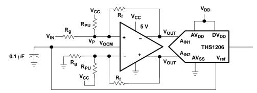
Figure 32. Circuit With Improved Common-Mode Input Voltage
