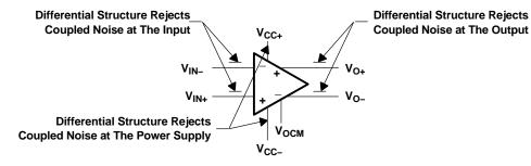
Figure 36. Definition of the Fully Differential Amplifier
