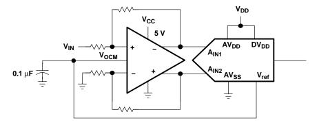
Figure 31. Fully Differential Amplifier Using a Single Supply
