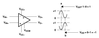
Figure 39. Fully Differential Amplifier With Two 1-V<sub>PP</sub> Signals
