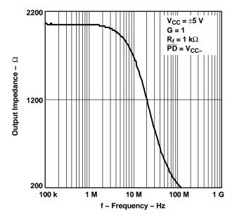
Figure 42. Output Impedance (In Power Down) vs Frequency
