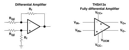
Figure 35. Differential Amplifier Versus a Fully Differential Amplifier
