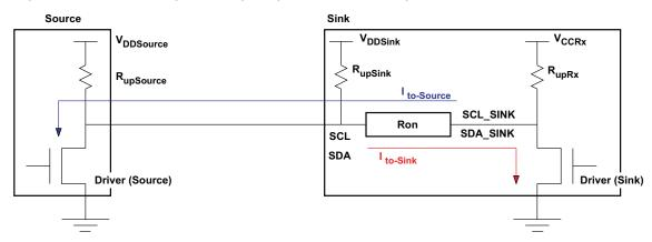
Figure 17. Simplified Electrical Circuit Model for DDC Channel
