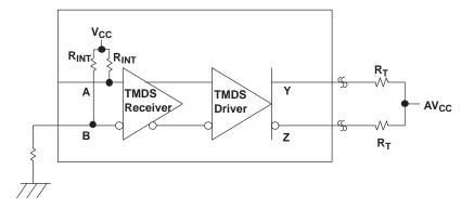
Figure 16. TMDS Input Fail-Safe Recommendation
