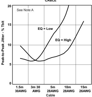
A. 1080p 12-Bit,  $V_{CC}=AV_{CC}=3.3$  V,  $T_A=25^{\circ}C$ ,  $R_{VSADJ}=4.02$  k $\Omega$ , See Figure 6, Clock Channel = 222.8 MHz, Data Channel = 2.228 Gbps
