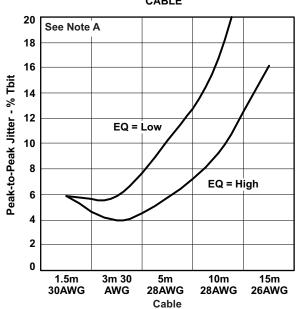
A. 1080p 10-Bit,  $V_{CC}=AV_{CC}=3.3$  V,  $T_A=25^{\circ}C$ ,  $R_{VSADJ}=4.02$  k $\Omega$ , See Figure 6, Clock Channel = 185.6 MHz, Data Channel = 1.856 Gbps
