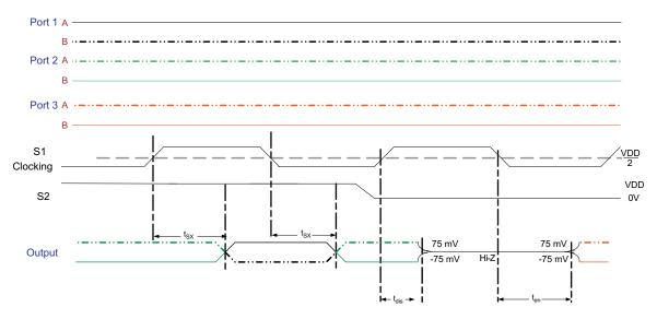
Figure 6. TMDS Outputs Control Timing Definitions
