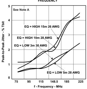
A. Channel 1,  $V_{CC} = AV_{CC} = 3.3$  V,  $T_A = 25^{\circ}C$ ,  $R_{VSADJ} = 4.02$  k $\Omega$ , See Figure 6 Figure 11.
