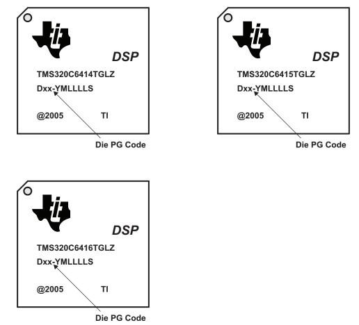
A NOTE: Qualified devices are marked with the letters "TMS" at the beginning of the device name, while non-qualified devices are marked with the letters "TMX" or "TMP" at the beginning of the device name.
