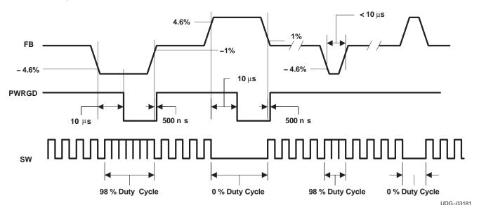
Figure 7. Duty Cycle Waveforms
