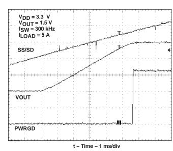
Figure 23. Start-Up Operation With Transient Comparators
