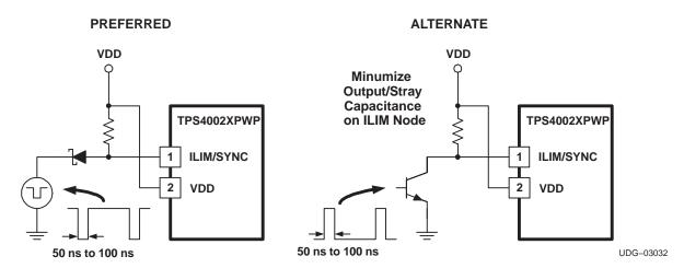
Figure 6. Synchronization Methods
