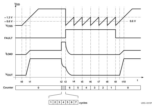
Figure 4. Overcurrent/Fault Waveforms
