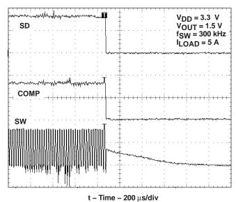
Figure 24. COMP Shutdown Operation
