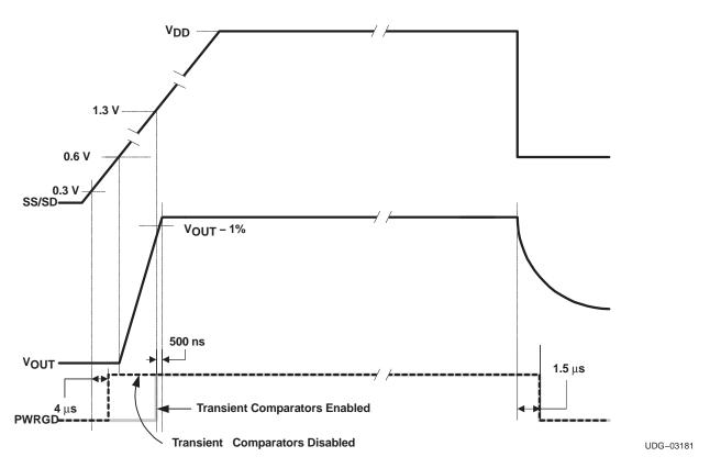
Figure 8. Transient Comparator Waveforms
