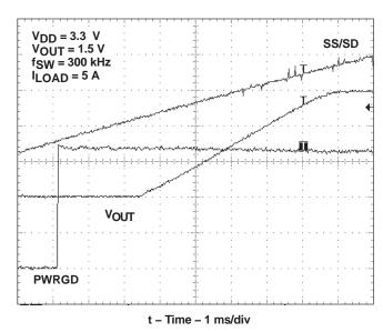
Figure 21. Start-Up Operation Without Transient Comparators
