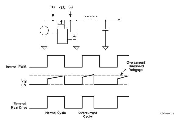
Figure 3. Switch Node Waveforms for Synchronous Buck Converter
