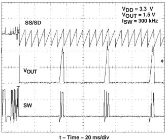
Figure 20. Output Current Fault Operation
