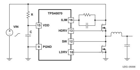
Figure 1. Limiting the Slew Rate
