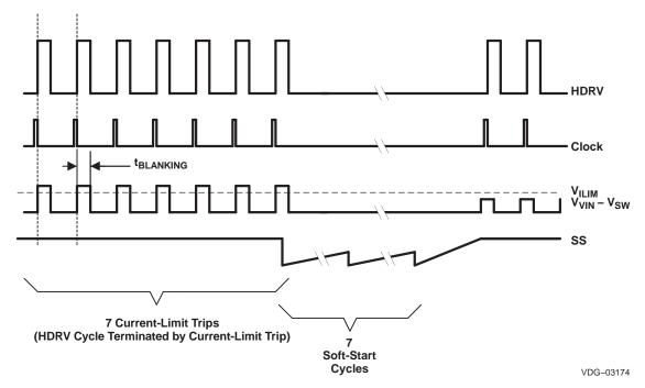
Figure 11. Typical Fault Protection Waveforms
