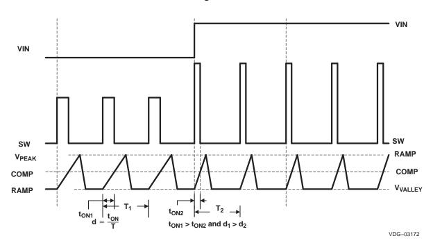
Figure 9. Voltage Feed-Forward and PWM Duty Cycle Waveforms
