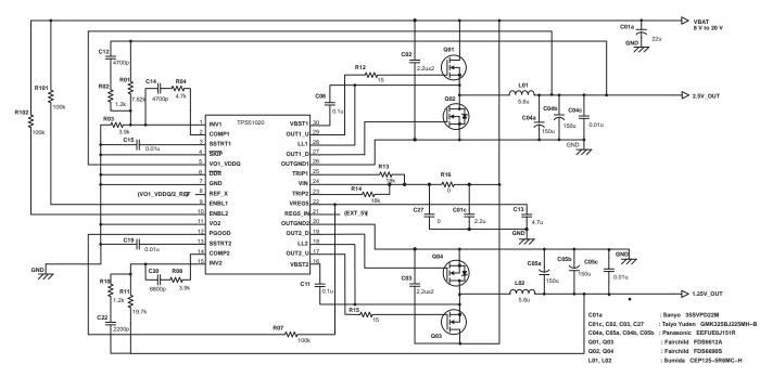
Figure 6. Typical Application Circuit: DDR(2.5V/6A + 1.25V/6A) from VBAT
