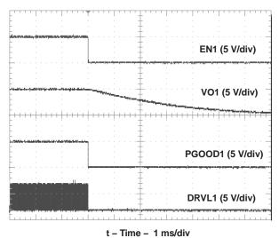
Figure 37. 5-V Soft-Stop Waveforms
