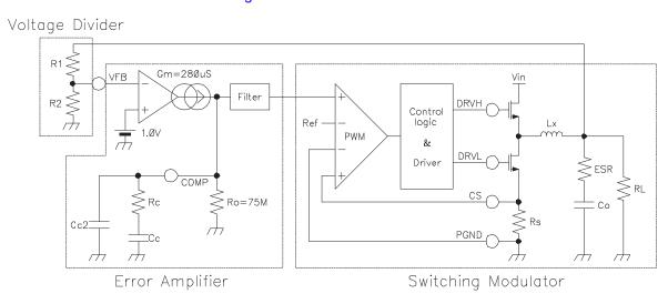
Figure 1. Linearizing the Modulator
