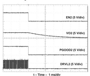
Figure 38. 3.3-V Soft-Stop Waveforms
