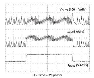
Figure 32. 3.3-V Load Transient Response
