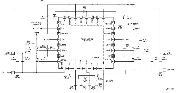
Figure 3. D-CAP™ Mode, Fixed 5-V/6-A, +3.3-V/6-A, R<sub>DS(on)</sub> Sensing
