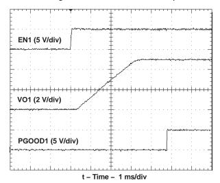
Figure 33. 5-V Startup Waveforms
