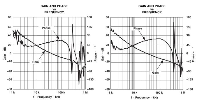
Figure 39. 5-V Bode Plot (Current Mode)
