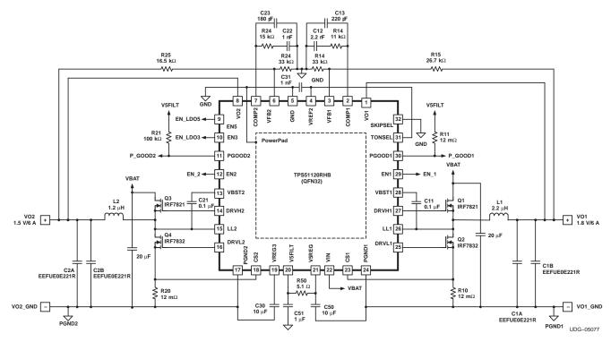
Figure 4. Current Mode, External 1.8-V/6-A, +1.5-V/6-A, R<sub>SENSE</sub> Sensing
