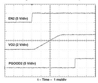
Figure 34. 3.3-V Startup Waveforms
