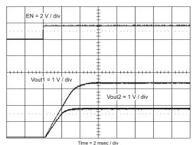
Figure 24. Ratiometric and Simultaneous Startup Figure 25. Ratiometric Startup With Vout1 Leading Vout2
