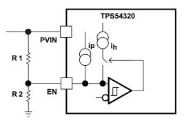
Figure 18. Adjustable PVIN UVLO, VIN  $\ge$  4.5 V
