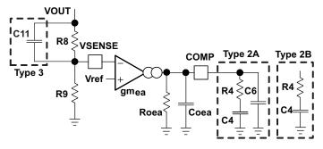
Figure 31. Types of Frequency Compensation
