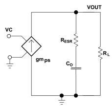
Figure 29. Simplified Small Signal Model for Peak Current Mode Control
