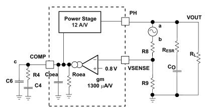
Figure 28. Small Signal Model for Loop Response
