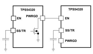
Figure 20. Sequential Start-Up Sequence
