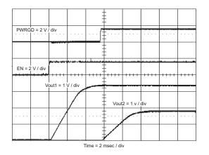
Figure 21. Sequential Start-Up Using EN and PWRGD
