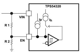
Figure 17. Adjustable VIN UVLO
