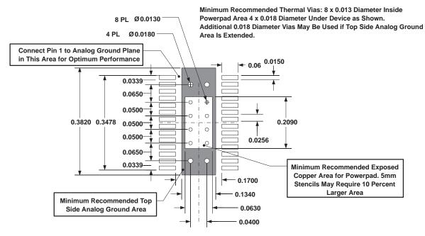
Figure 11. Recommended Land Pattern for 28-Pin PWP PowerPAD
