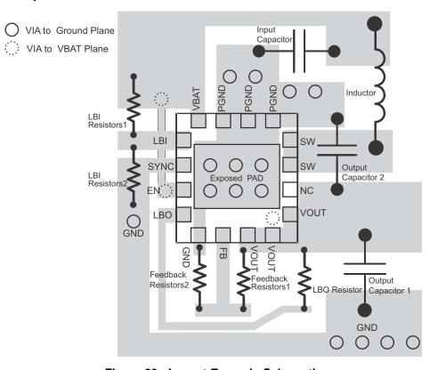
Figure 23. Layout Example Schematic
