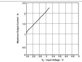
Figure 1. TPS61091 Maximum Output Current vs Input Voltage
