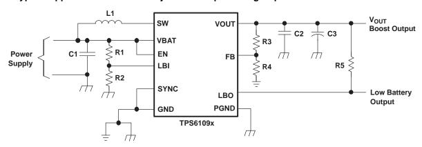
Figure 14. Typical Application Circuit for Adjustable Output Voltage Option Schematic
