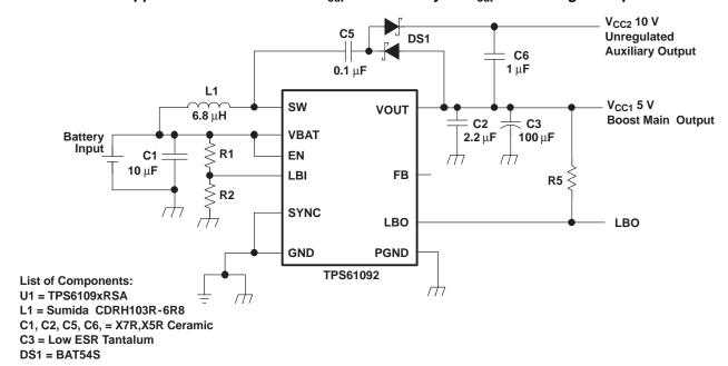
Figure 21. Power Supply Solution With Auxiliary Positive Output Voltage Schematic
