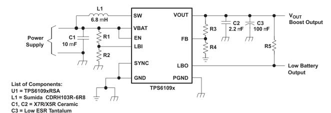
Figure 13. Parameter Schematic
