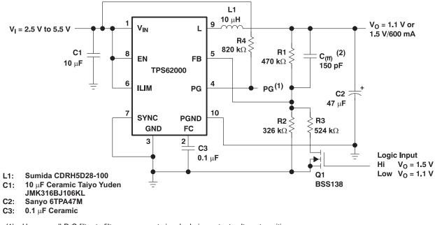
(1) Use a small R-C filter to filter wrong reset signals during output voltage transitions.
