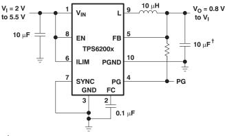
$^{\dagger}$  With V\_O  $\geq$ 1.8 V; C\_o = 10  $\mu$ F, V\_O <1.8 V; C\_o = 47  $\mu$ F
