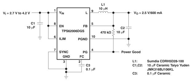
Figure 18. Single Li-ion to 2.5 V/600 mA Using Ceramic Capacitors Only
