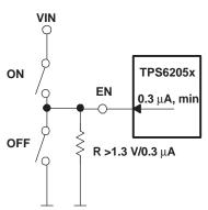
Figure 19. Pushbutton Configuration for the EN-Pin
