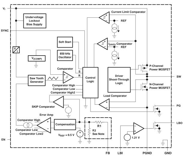
NOTE: For the adjustable versions (TPS62050, TPS62051), the internal feedback driver is disabled and the FB pin is directly connected to the GM amplifier.
