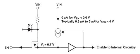
Figure 18. Internal Circuit of the ENABLE Pin
