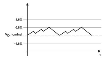
Figure 17. Power-Save Mode Output Voltage Thresholds
