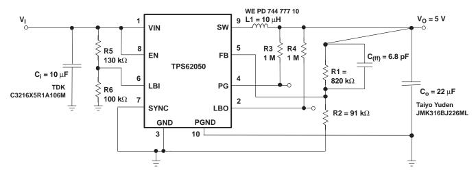
Quiescent Current Measurements and Efficiency Were Taken With: R5 = Open, R4 = Open, LBI Connected to GND.
