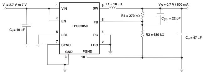
The TPS62050 is used to generate output voltages as low as 0.7 V. With such low output voltages, the inductor discharges very slowly. This leads to a high output voltage ripple in power-save mode (SYNC = GND). It is therefore recommended to use a larger output capacitor to keep the output ripple low. With an output capacitor of  $47 \, \mu F$ , the output voltage ripple is less than  $40 \, \text{mV}_{PP}$ .
