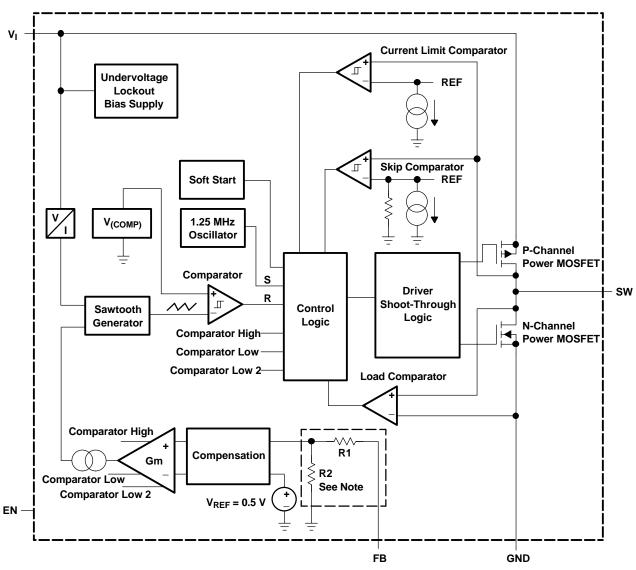
NOTE: For the adjustable version (TPS62220) the internal feedback divider is disabled, and the FB pin is directly connected to the internal GM amplifier
