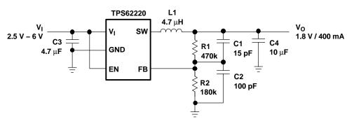
Figure 15. Typical Application Circuit for the TPS62220 With Adjustable Output Voltage
