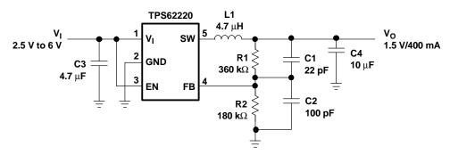
Figure 20. LI-Ion to 1.5-V Conversion
