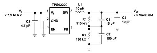
Figure 18. LI-Ion to 2.5-V Conversion
