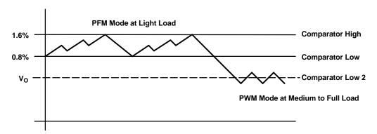
Figure 14. Power-Save Mode Thresholds and Dynamic Voltage Positioning
