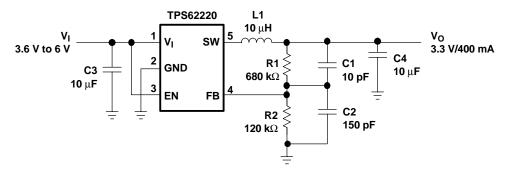
Figure 17. LI-Ion to 3.3-V Conversion
