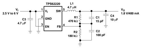
Figure 19. LI-Ion to 1.8-V Conversion
