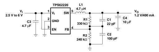
Figure 21. LI-Ion to 1.2-V Conversion
