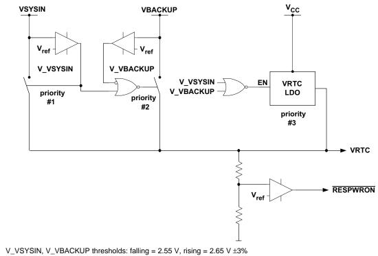
B. **RESPWRON** thresholds: falling = 2.4 V, rising =  $2.52 \text{ V} \pm 3\%$
