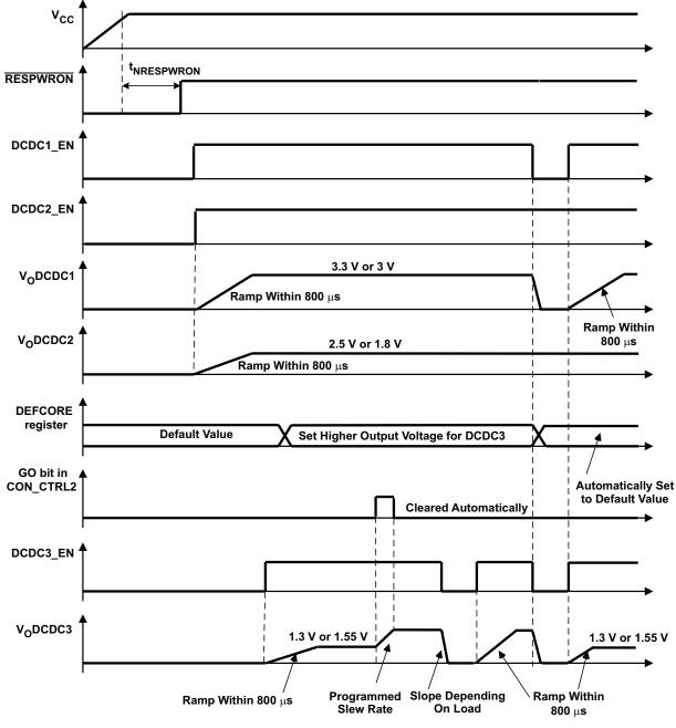
Figure 28. DVS Timing
