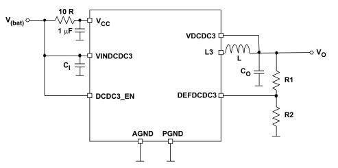
Figure 35. External Resistor Divider
