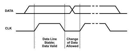
Figure 29. Bit Transfer on the Serial Interface
