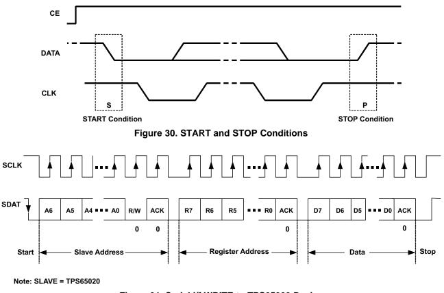
Figure 31. Serial i/f WRITE to TPS65022 Device
