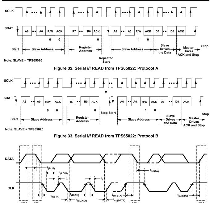
Figure 34. Serial i/f Timing Diagram
