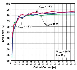
Figure 18. LED DRIVER EFFICIENCY vs OUTPUT CURRENT
