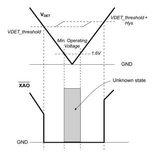
Figure 31. Voltage Detection and  $\overline{XAO}$  Pin
