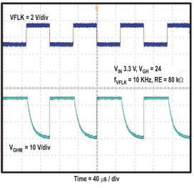
Figure 15. GATE VOLTAGE SHAPING
