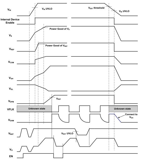
Figure 32. Power Up/Down Sequence
