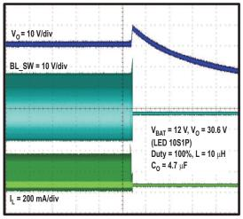
Time = 400 ms / div Figure 24. LED DRIVER OPEN WLED PROTECTION
