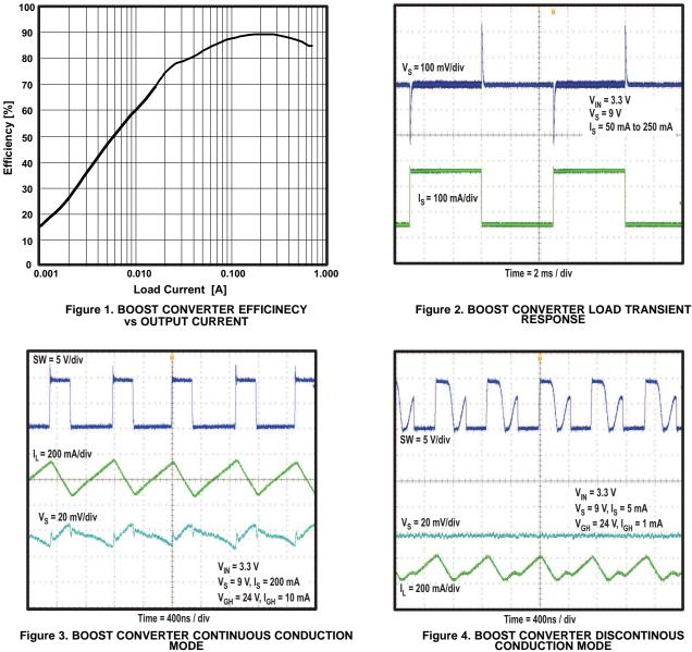
Figure 4. BOOST CONVERTER DISCONTINOUS CONDUCTION MODE
