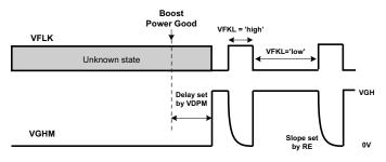
Figure 30. Gate Voltage Shaping Timing
