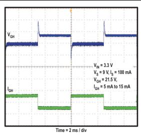
Figure 6. POSITIVE CHARGE PUMP LOAD TRANSIENT RESPONSE
