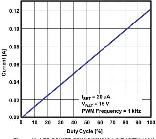
Figure 19. LED DRIVER PWM DIMMING LINEARITY 100Hz
