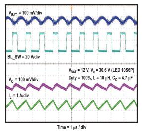
Figure 21. LED DRIVER SWITCHING WAVEFORM
