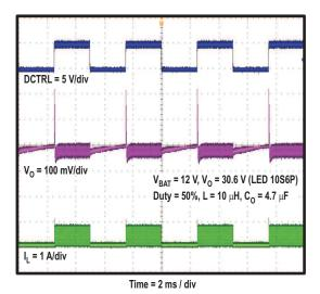
Figure 22. LED DRIVER OUTPUT RIPPLE AT PWM DIMMING
