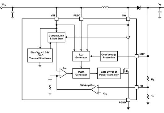
Figure 25. Boost Converter Block Diagram
