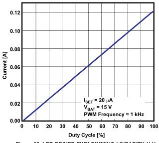
Figure 20. LED DRIVER PWM DIMMING LINEARITY 1kHz
