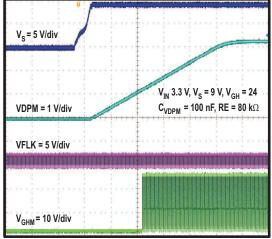
Time = 4 ms / div Figure 13. POWER ON SEQUENCE OF VGHM
